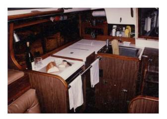
L-shaped galley with 3-burner propane stove with oven and broiler. Gas warner and Marinetic gas shutoff valve. Excellent galley storage and working area with worktop cover for stove. Extensive storage possibilities and galley equipment. Fridge 225 litre.
